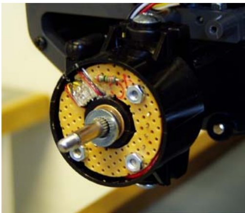
Figure 2.4: HEDR-8000 in the wheel house attached to a piece of print.
